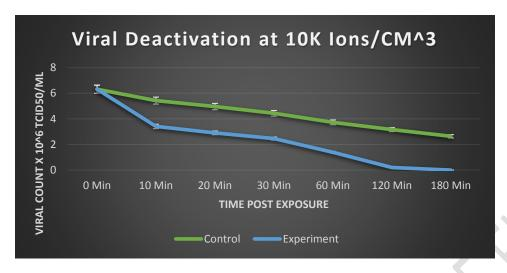
Log 10 Reduction 10 Min: 0.27, 20 Min: 0.34, 30 Min: 0.41, 60 Min: 0.66, 120 Min: 1.49, 180 Min: 3.94
